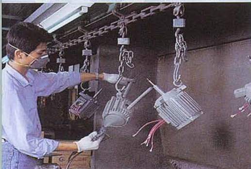
Electrostatic coating, low temperature painting
