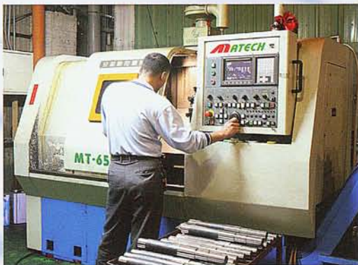
CNC lathing of shaft spindles
