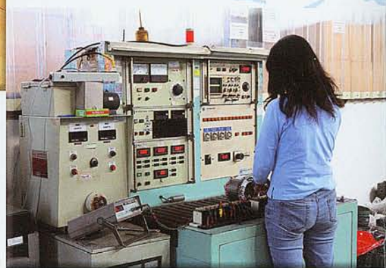
Computerized Testing of Coiled Stator
